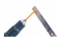
How to cut stick types: Make notches from both sides using an electrodeposited diamond file and cut off a tip.
