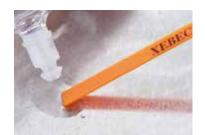
Applying lubricant improves polishing efficiency. \*Using a metal lubricant is recommended.
